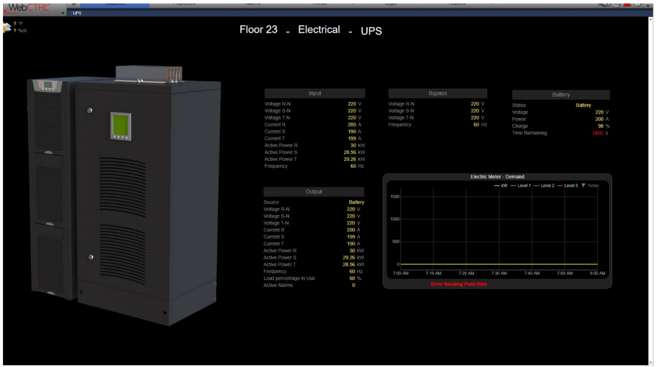
Figure 3: IDCAM provides insight into the existing battery life on a UPS and can sufficient warning time in advance of failure for workloads to be properly and safely migrated – WebCTRL® building automation system.
