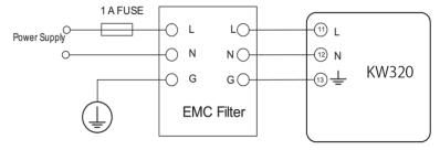
Choice of wire of power supply is AWG 22-16 or 0.6-1.5 mm2.
