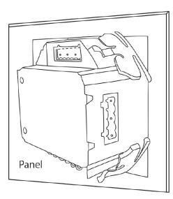
**NOTE** The display meter and the remote display unit have the same installation method. The DIN rail meter is simply installed on a 35mm DIN rail.
