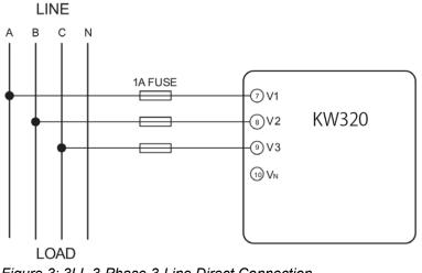
Figure 3: 3LL 3-Phase 3-Line Direct Connection
