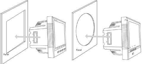
3. Install clips on the back side of the meter and secure tightly to ensure the meter is affixed to the panel.
