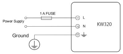
A fuse (typical 1A/250VAC) should be used in the auxiliary power supply loop. No. 13 terminal must be connected to the ground terminal of the switchgear. An isolated transformer or EMC filter should be used in the control power supply loop if there is a power quality problem in the power supply.
