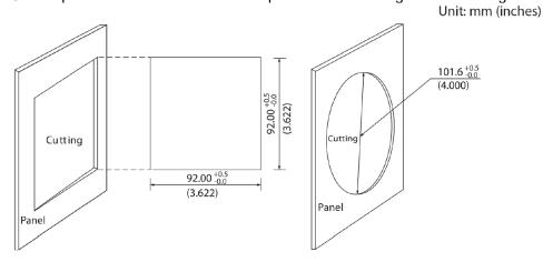
2. Remove the clips from the meter and insert the meter into the square hole from the front side. Please note: optional rubber gasket must be installed on the meter before inserting the meter into the cut out.
