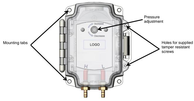
Figure 1: Differential Pressure Switch
