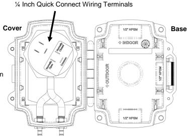
**Figure 4:** Pressure Switch Open Showing Switch Connections
