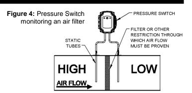
To set the pressure trip point, remove the tubing from the
