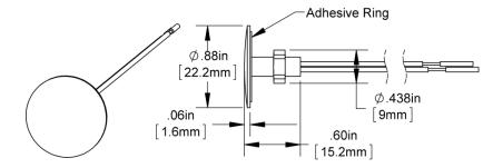
Figure 1: Low Profile Button Sensor Part numbers: NSB-10K-2-LPW NSB-50K-LPW
