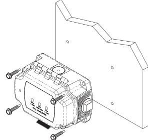
Figure 4: Mounting the Rough Service sensor to a wall
