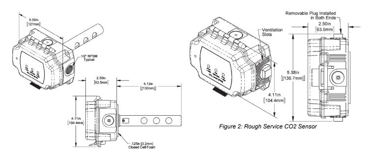
Figure 1: Duct CO2 Sensor
