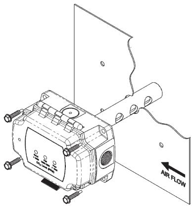
Figure 5: Duct unit mounting
