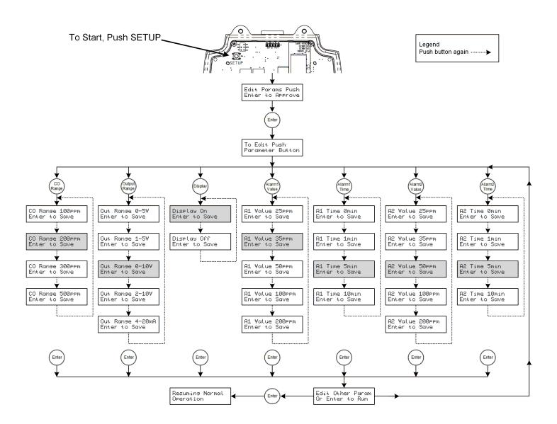
**Figure 19: P**arameter Setup Flow Chart (Default settings are shown with gray shading)
