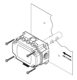
Figure 4: Duct unit mounting
