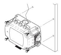
Figure 3: Rough service unit mounting
