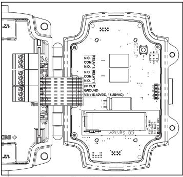
Figure 5: Field Wiring Terminals
