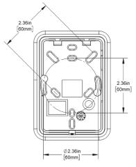
Fig. 4: 60mm mounting base dimensions
