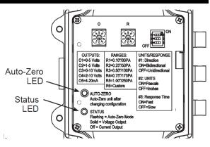
Figure 5: Auto-Zero and Status LEDs
