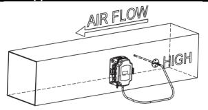
Figure 7: Duct Static Pressure Monitoring (ZPM Pressure Sensor mounted on the duct with a Static Pressure Probe in the duct.)
