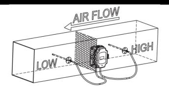
Figure 8: Air Filter Pressure Drop Monitoring (ZPM Pressure Sensor mounted on the duct with a Static Pressure Probe on either side of the filter in a duct.)
