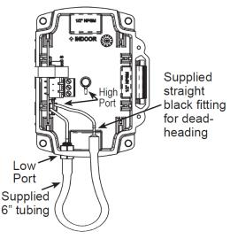
Figure 6: Deadheading ports on units with attached tube
