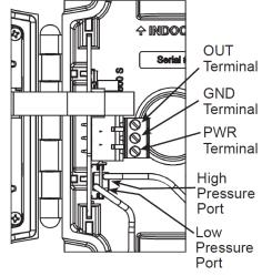
Figure 4: ZPM Wiring Terminals
