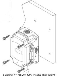
Figure 1: BBox Mounting (for units without Attached Tube option)
