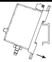
Figure 2: Catch the EZ mount hook on the edge of the DIN Rail, then rotate into place
