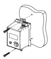
Figure 4: Surface Mounting with Tabs Out
