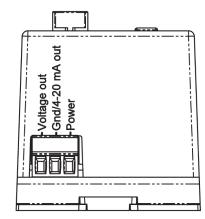
Figure 6: Wiring Terminations
