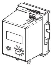
Figure 3: Snaptrack Mounting with Tabs In
