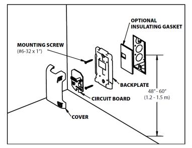
Figure 2: Mounting Diagram
