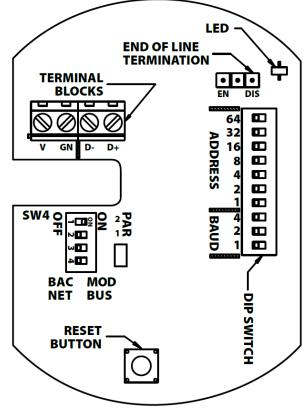
Figure 3: Wiring Diagram
