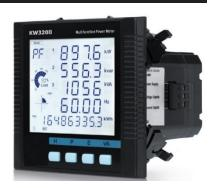
Active Power, Reactive Power and Apparent Power – see table 1 for all parameters monitored and metered. Current input are compatible with a 333mV and Flexible Rogowski Coil CT. Meters come standard with a three channel CT input to accurately measure neutral current. CTs are sold separately as shown on the Split-Core, Solid-Core and Rogowski Current Transformer product data sheets.
