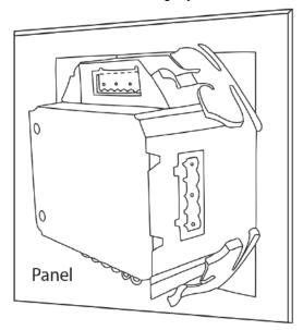
Figure 4: Use the clips to fix the meter on the panel
