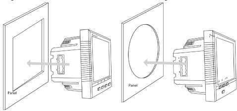
Figure 3: Put the meter in the opening
