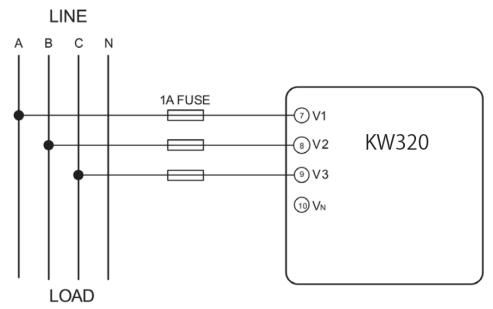
Figure 10: 3LL 3-Phase 3-Line Direct Connection
