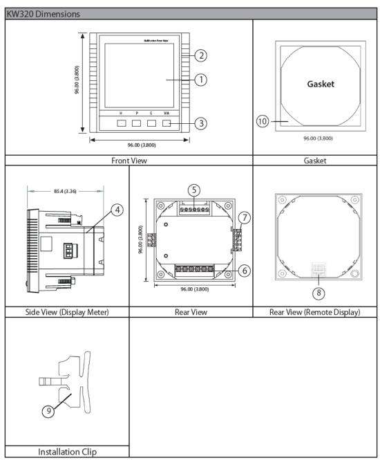
Figure 1: Dimensions and Part Names
