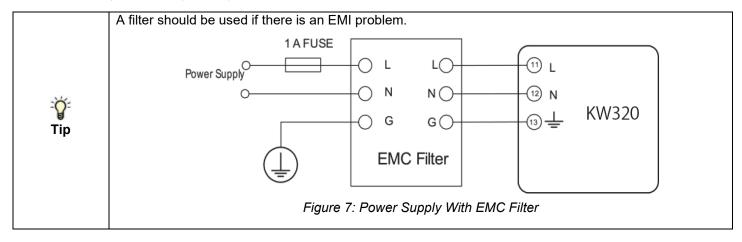
Choice of wire of power supply is AWG 22-16 or 0.6-1.5 mm2.
