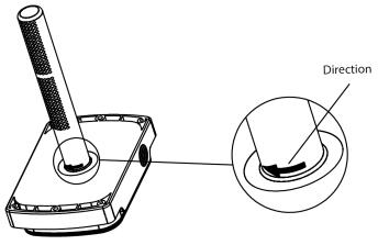
Figure 5: Attaching Sample Probe
