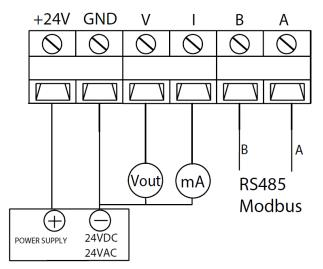
Figure 8: Wiring
