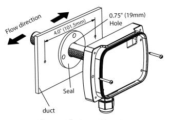
Figure 7: Enclosure Mounting
