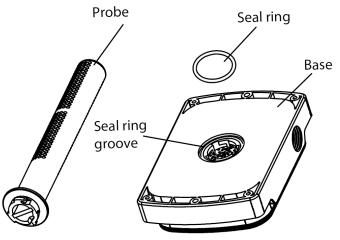
Figure 2: Duct Components
