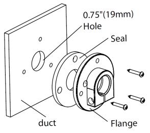
Figure 3: Flange and Seal Installation
