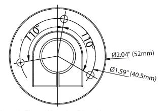
Figure 6: Flange Mounting Dimensions
